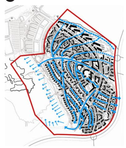
Urriðaholt sustainable drainage system - green wedges provide retention for severe storm events
